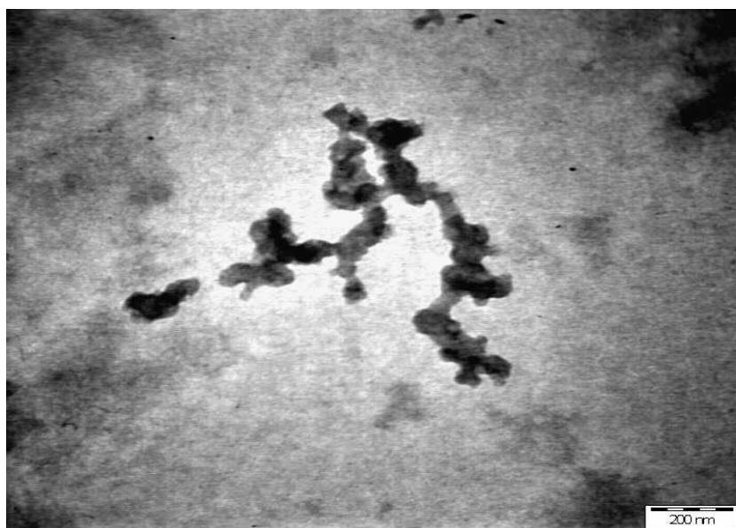
*Figure 4.57: Transmission electron micrographs of negatively stained preparations from LBS granules treated with  $H_2SO_4$  at  $40^\circ C$  under continuous stirring (200 nm)*
